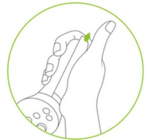
Slide the battery cover according to arrow direction with your palm.
